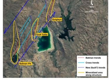
Figure 1 – Relationship of known structural trends relative to existing mineral deposits and exploration targets.
