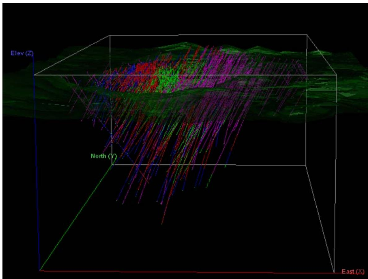
**FIGURE 17-11: Drilling Pattern, looking north shown with GEMCOM software.**
