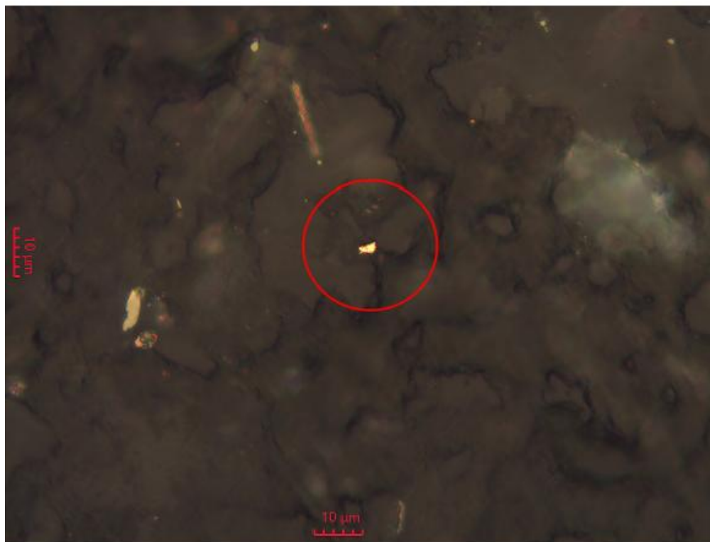
Client Sample No.: Mt. Todd BYellow Small 3μm grain of Au sits between quartz grains – 500X RL
